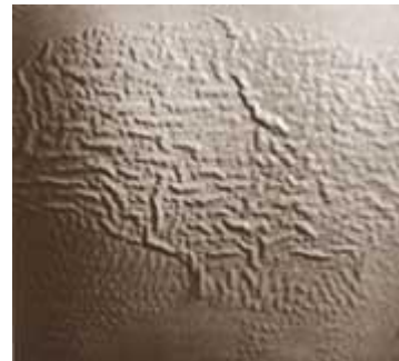
Wrinkled layers can generally be removed by scraping and sanding as opposed to total paint removal. Photo: Courtesy, National Decorating Products Association.
